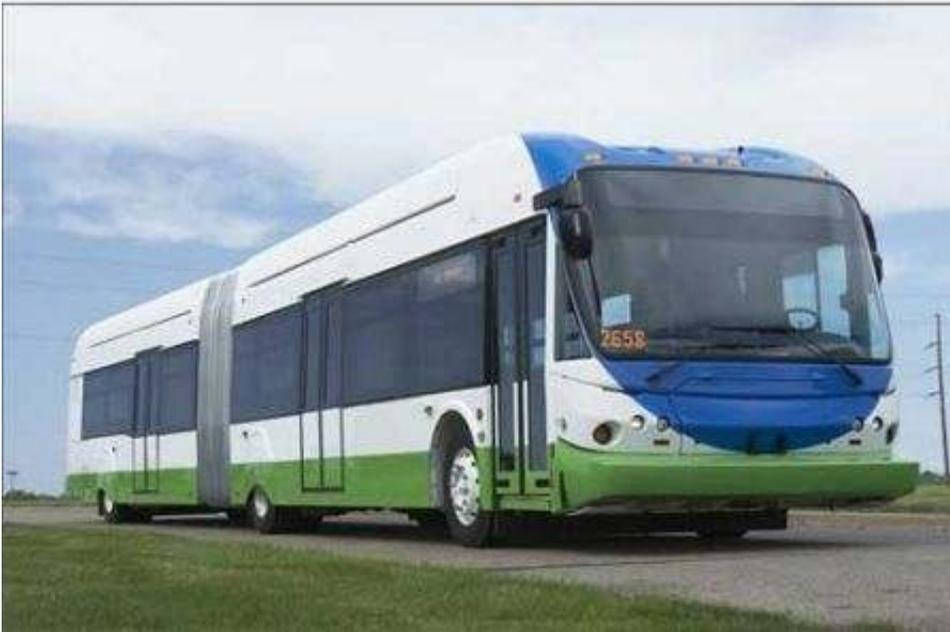
Hybrid transit bus systems resemble the passenger vehicle systems with the exception of size. The high-voltage batteries are usually NiMH (nickel metal hydride) and are placed on the roof of the bus. They, therefore, are away from the passenger area. System voltages are in the 800-volt range. The high-voltage orange cables in transit buses run down the rear corner of the bus to the propulsion control system. Note the location of the battery housing on the roof in the photo below.
