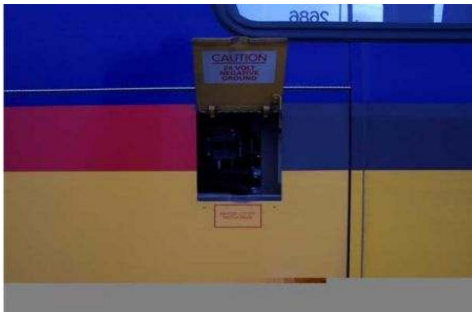
The switch is usually labeled “ON” and “OFF.” Note that this switch from a New Flyer Hybrid Bus (below) is mounted upside down. In this case, the switch is labeled “NO” and something that might be a foreign language.
